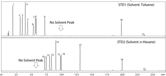
Fig. 2 Chromatograms of 19 Sulfur Compounds (10 ppm)
