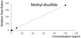
Fig. 3 Calibration Curve for 2-Propanethiol and Methyl Disulfide
